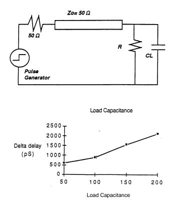
The following diagram illustrates the change in delay readings when a capacitive element is introduced into the middle of the ideally-matched cable.
