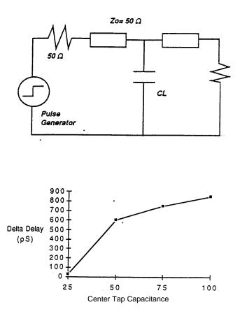
The following diagram illustrates an actual series of measurements, showing the delay in cable measurement that results from placing a cable of mismatched impedance in a test setup.
