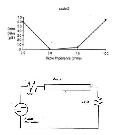
The following diagram illustrates the change in delay readings when the terminating impedance is mismatched.
