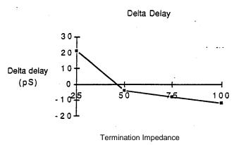
The following diagram illustrates the change in delay readings when the terminating capacitance is mismatched.
